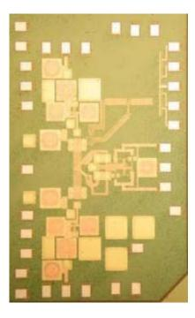
24 GHz receiver 2 channels Analog baseband phase rotation ESSCIRC 2010
