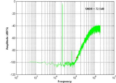
Simulated output spectrum of the delta-sigma modulator
