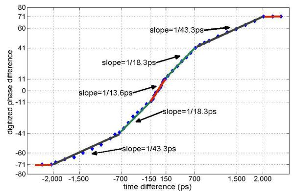
Measured characteristic of Uneven-cell TDC
