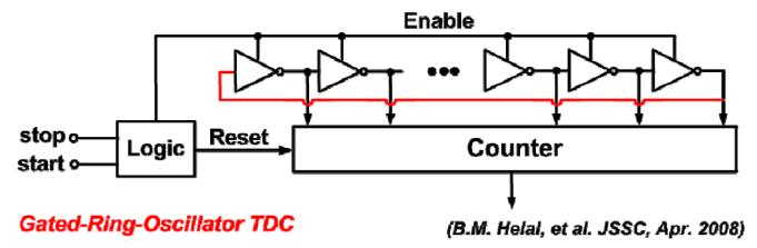
However, coarse resolution still limited by an inverter delay
