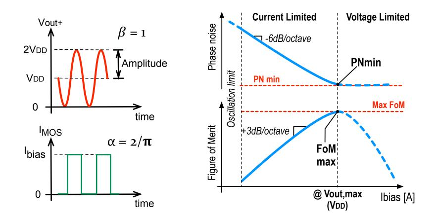
With  $Q_t$ = 13, the Class-B oscillator has an ideal maximum FoM of 194dBc/Hz
