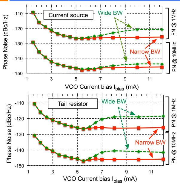
The narrow loop bandwidth filters the opamp noise when the VCO starts working in class-B
