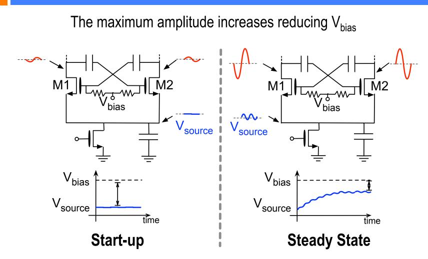
The start-up condition limits the lower value of V<sub>bias</sub>
