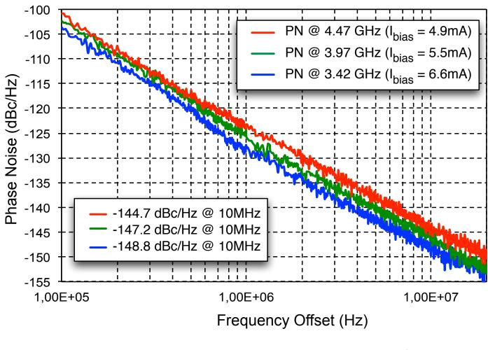
With  $I_{bias} = 5.5 \text{mA}$ , FoM = 191dBc/Hz
