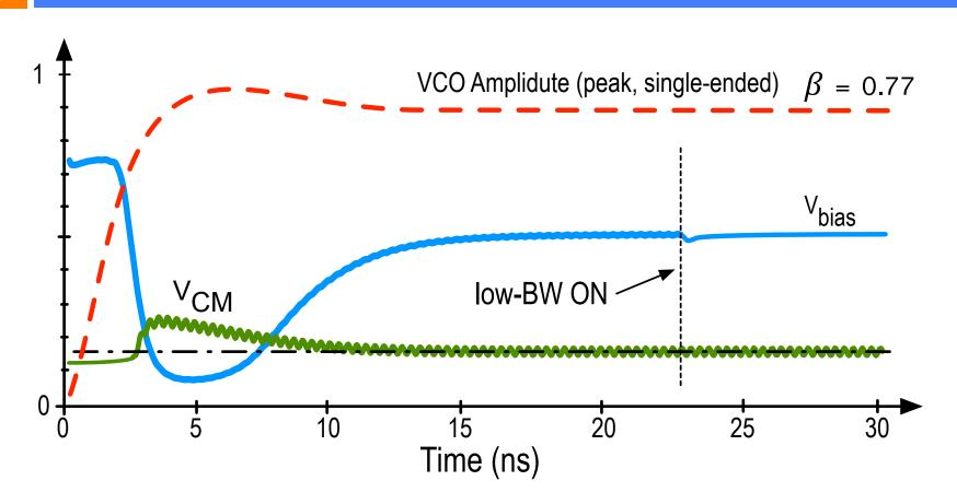
The low feedback-generated  $V_{bias}$  maximizes the oscillation amplitude, optimizing the phase noise performance
