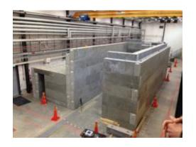
Bunker in Uppsala in which accelerating cavities will be tested att 300 kW power and at 2K.
