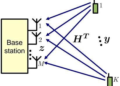
Down-link:  $m{y}=m{H}m{z}+m{n}$  Up-link: $oldsymbol{z} = oldsymbol{H}^Toldsymbol{y} + oldsymbol{v}$
